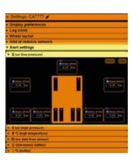
Configure all settings including wheel layouts and numbering, alarm levels and sensor changes.
